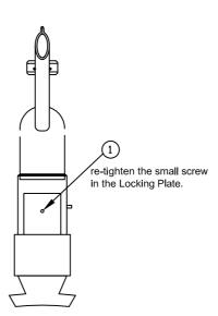
5. Rotate Dryer or Processor to check that it turns smoothly through 360 degrees before re-tightening screw in Locking Plate [1]. The Locking Wedge is now held securely, preventing the Dryer or Processor from dropping out of the Pivot Hood.
