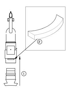
3. Insert Swivel Boss of Dryer or Processor into Pivot Hood [1], lining up the groove in the Boss with the slot in the Hood and place the Locking Wedge in position [2].
