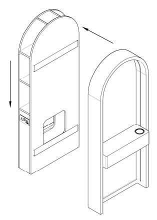
3. Connect electrical / power cables before completing this procedure: Carefully place Halo Styling Unit (B) against Island Column (A) Ease down until the wall unit locks into position and is secure.
