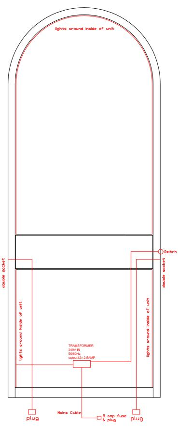
The Halo Island Unit is supplied with LED light feature. These lights must be installed, inspected, and tested by qualified personnel to meet the Requirements for Electrical Installations, IEE Wiring Regulations, 17th Edition. Advice on further periodic inspection and testing should be sought from the technician carrying out the initial installation. Once installed, movement of the unit, modifications, repairs etc. should only be carried out in accordance with the contents of this notice.
