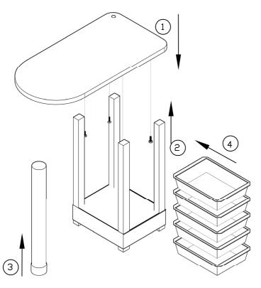
2. If the unit feels uneven, this can be corrected by turning the adjustable foot on the Leg (B).
