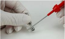
Use the brush to remove all dirt residues from the drill-hole of the chuck:
