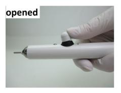
Now insert the tool as far as possible. Pull back the knob and the tool will be firmly clamped.
