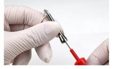
Rinse the chuck very well, and make sure you let it dry well afterwards. Cover your index finger with a very little amount (just a drop) of oil and rub in between your thumb and index finger. Dab off the oil until your fingers is only covered with a very thin film of oil. Now move the chuck in between your thumb and index finger. There should be only a very thin film of oil left on the chuck. Please act according to the saying: Less is more.
