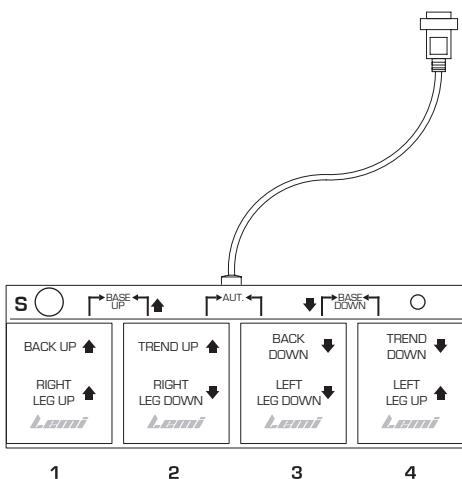
**!** To ACTIVATE the electric legs, press the **S BUTTON** (green LED on) BEFORE pressing any pedal.
